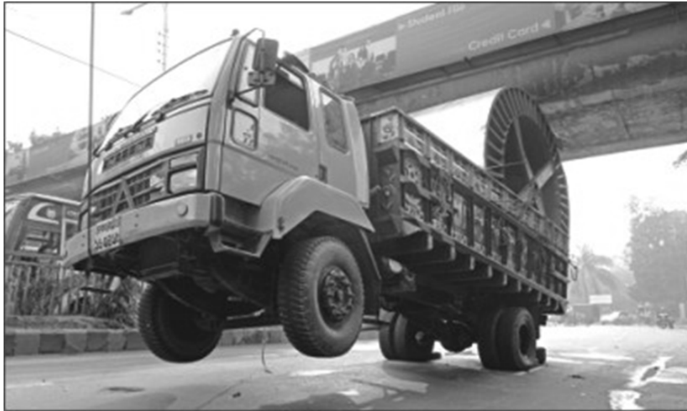
Figure 3: Over height Truck stuck with ramna footbridge
