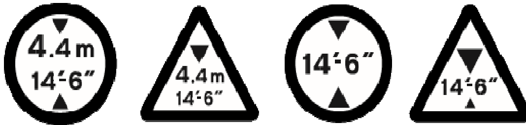
Figure 6: Traffic signs used at bridges to show the maximum permitted vehicle height
