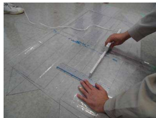
2) Heat welding polyolefin sheets
