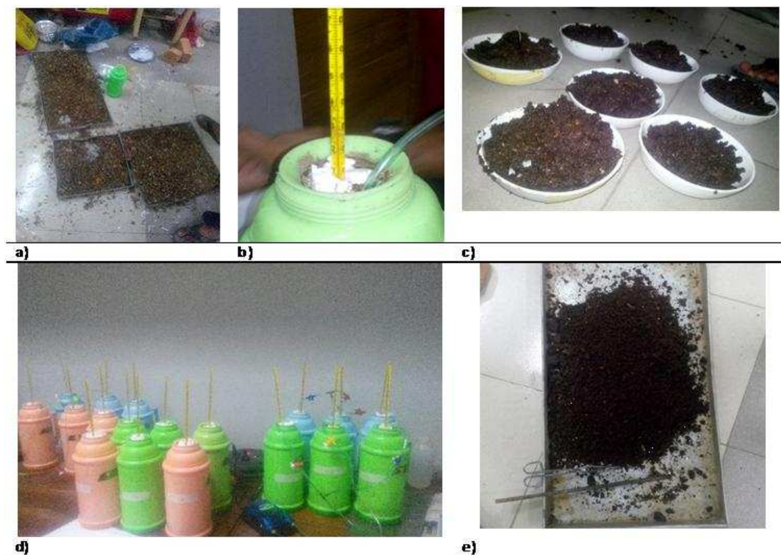
Figure 1: (a) Prepared waste mixture contains 60% moisture content approximately, (b) Thermometer and pipe were placed into the reactor; (c) Prepared waste mixture in porcelains before drying in oven, (d) Waste mixture in the reactor (Thermo flask) was covered by pieces of foam, (e) End product (compost) after ending of second stage.
