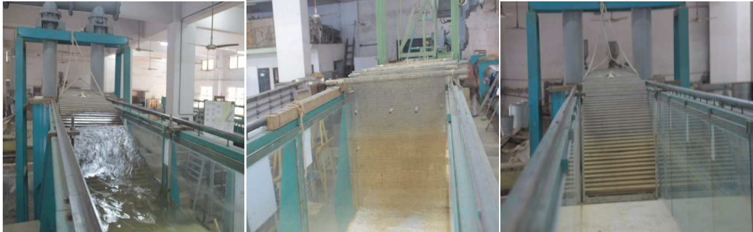
Figure 3: wire screen (1 st from the left); wave absorber (2 nd and 3 rd )
