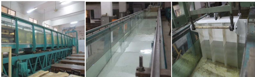
Figure 2: Laboratory Wave flume (1 st and 2 nd from the left); Wave Generator (3 rd one)
