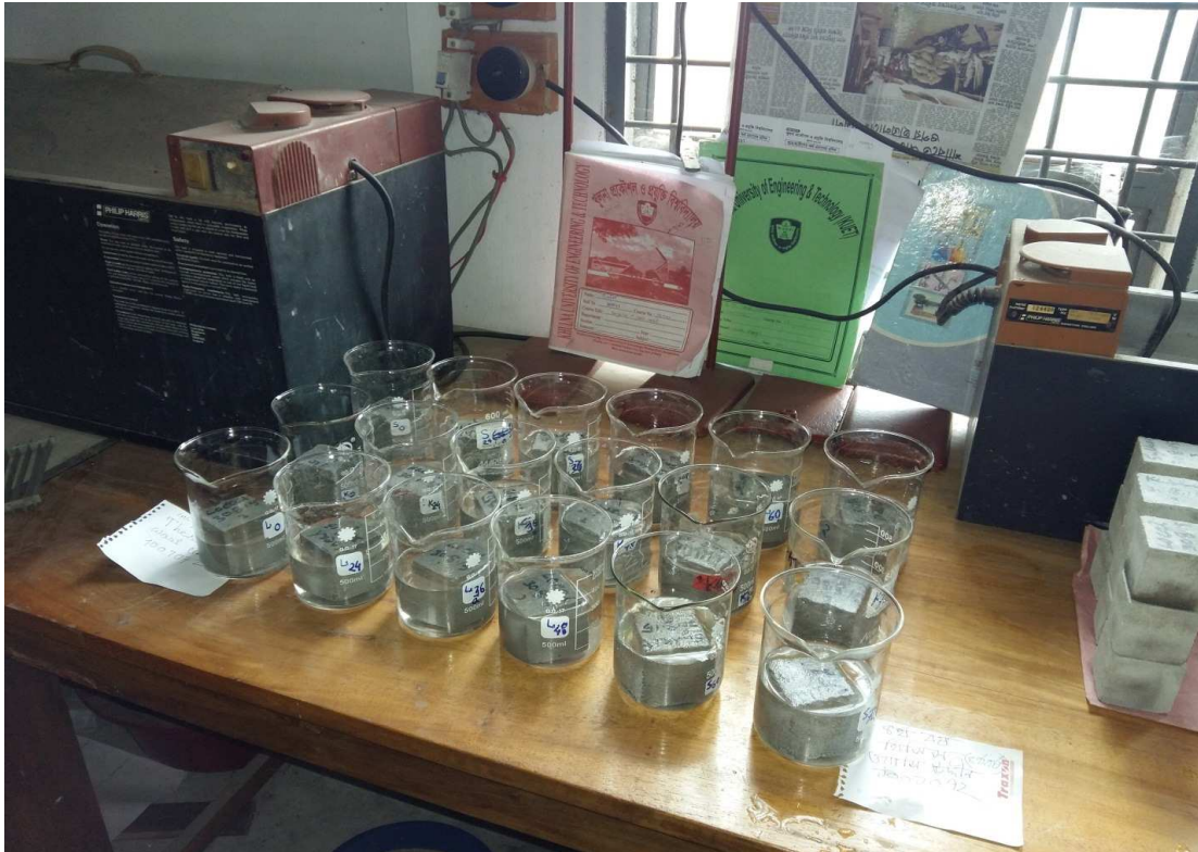
Figure 5: Soaking of 2" mortar cubes of Sylhet, Kushtia & Local sands for nine different durations
