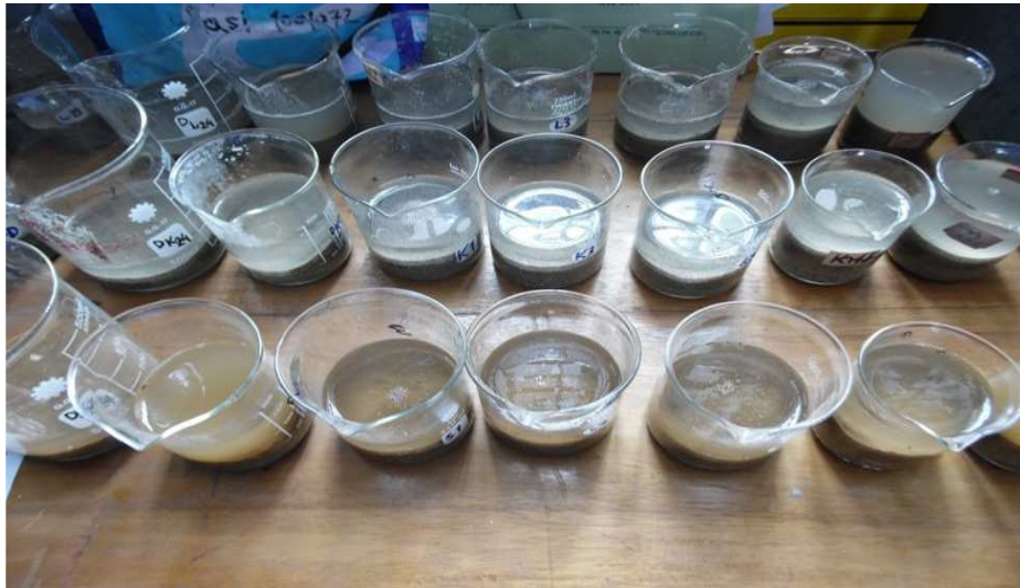
Figure 4: Soaking of Sylhet, Kushtia and Local sands for nine different time durations
