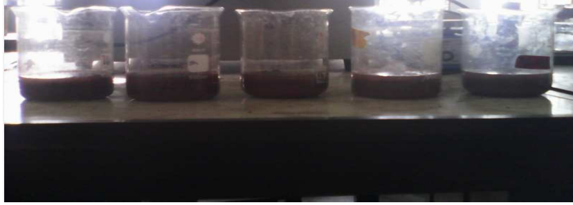
Figure 3: Soaking of brick aggregates for different time durations
