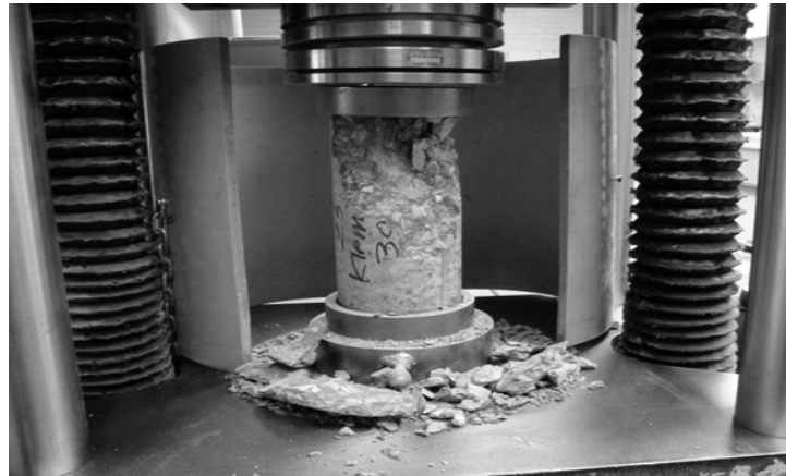
Figure 5: Determination of compressive strength of concrete
