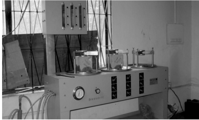
Figure 2: Placing the specimens on the permeability apparatus
