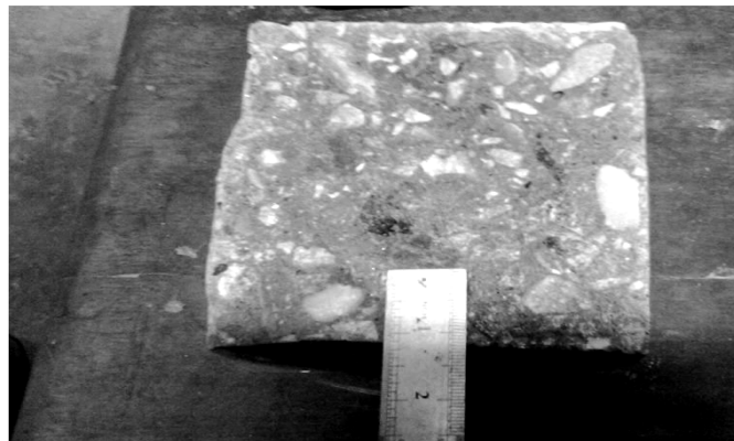
Figure 4: Measurement of depth of penetration
