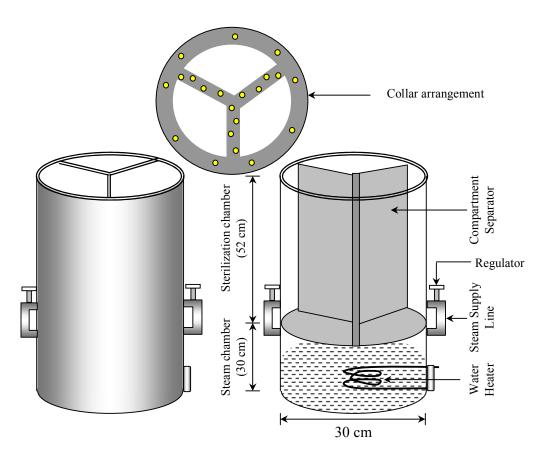
Figure 1: Schematic diagram of continuous operating autoclave
