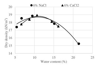
Figure 4: Comparison of dry density and water content of stabilized soils with chemical compounds at 6%.
