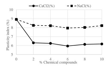
Figure 2: Comparison of PI of stabilized soils with chemical compounds.
