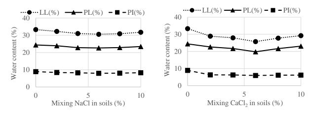
Figure 1: Effect of (a) NaCl and (b) Cacl<sub>2</sub> on Atterberg limits of stabilized soils
