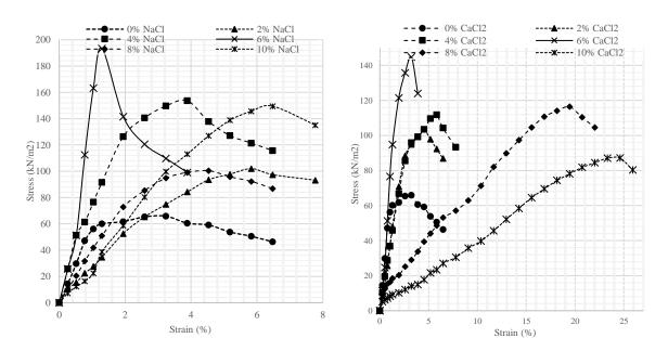
Figure 5: Effect of (a) NaCl and (b) Cacl<sub>2</sub> on unconfined compression strength of stabilized soils.
