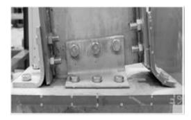
(a) Deformation of connection just after the test (Hasan et al., 2019)
