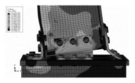
(b) Deformation of connection attained from FEA at the end
