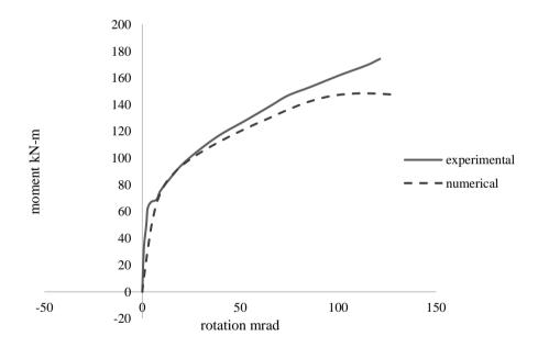
Figure 3: Verification of Moment-Rotation Curve between Experimental and FE model
