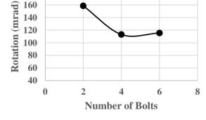
Figure 14: Moment vs Number of Seat Bolts in Beam curve
