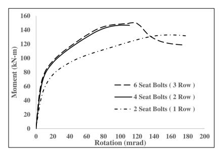
Figure 13: Moment vs Rotation Curve for Top-Seat Bolts in Beam Flange Analysis
