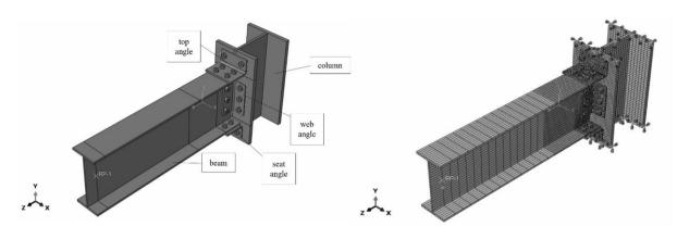
Figure 1: Details of joint
