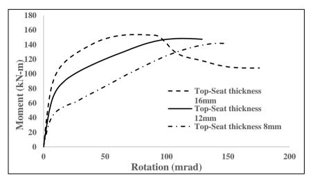
Figure 5: Moment-Rotation curve for top-seat angle thickness analysis
