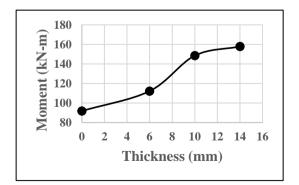
Figure 10: Moment-Thickness curve for Web angle thickness analysis
