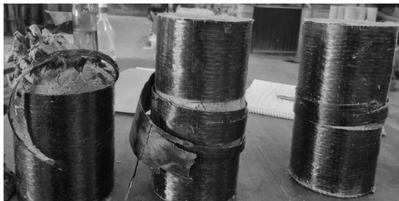
Figure 10: Failure pattern of cylinders wrapped in three layers
