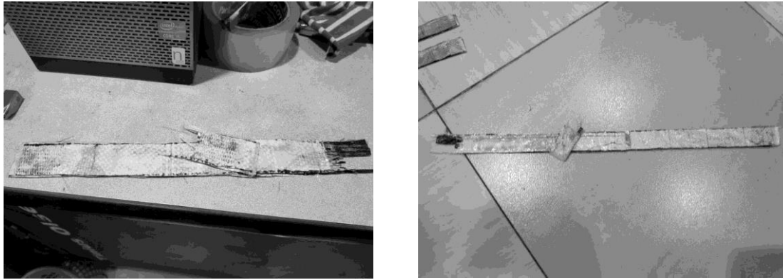
Figure 06: Typical failure pattern of flat tensile and overlap splice coupons
