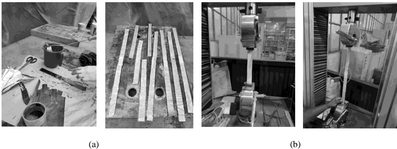
Figure 01: (a) Preparation and (b) Testing of Flat tensile and overlap splice coupons
