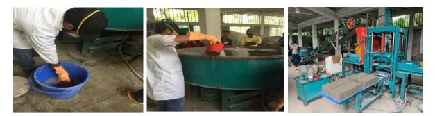
e) Mixing of water with SP-1 and SP-2. f) Mixing of SP-1 and SP-2 with other raw materials.
