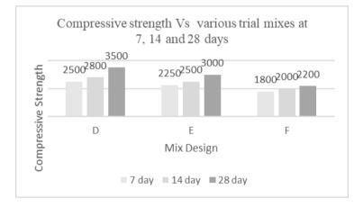
Figure -5: Compressive Strength of various sand cement block mixes at 7, 14, and 28 days.
