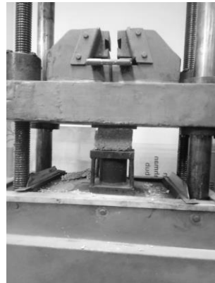
Figure 5: Compressive strength test of the sample.
