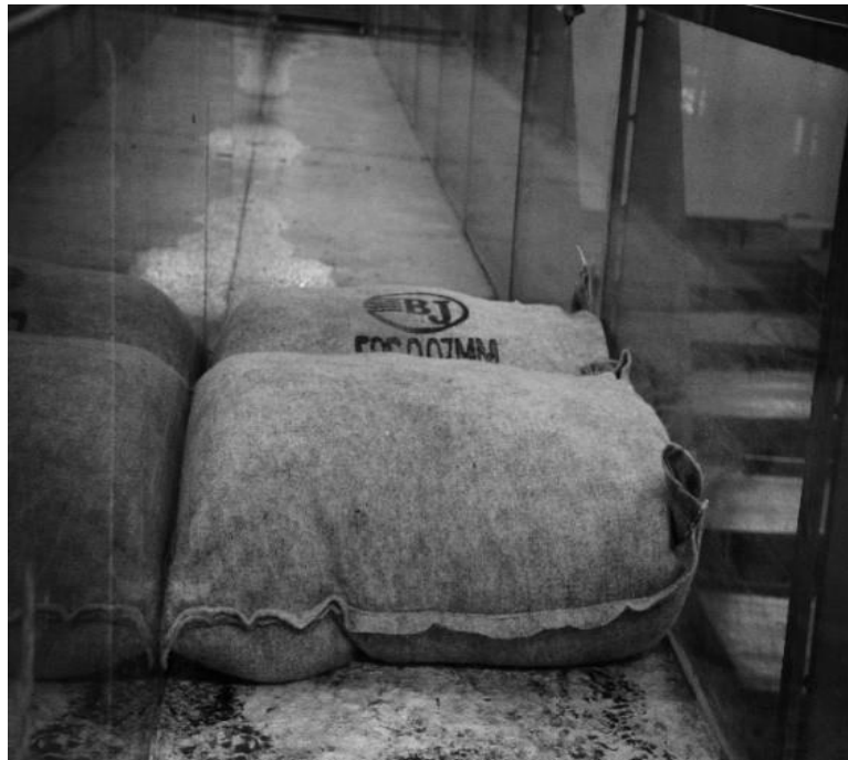
Figure 1(b): Geotextile tube filled with sand (Lateral View)
