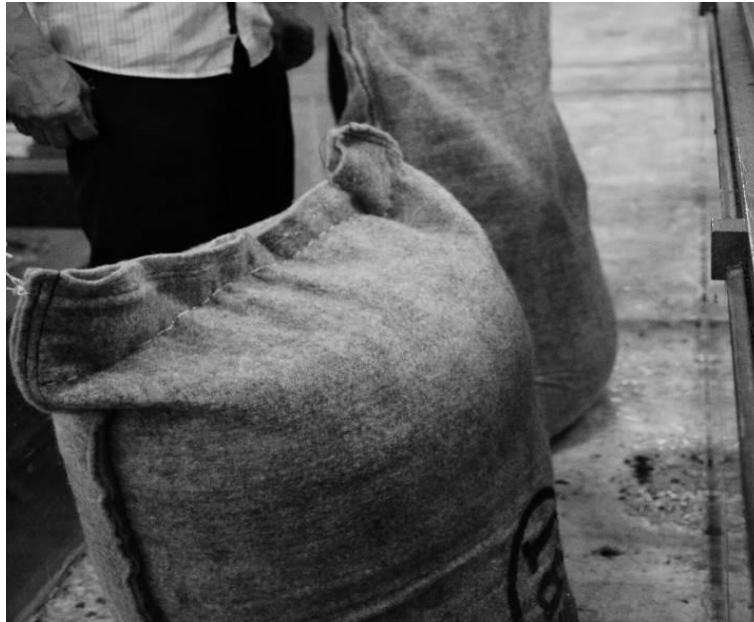
Figure 1(a): Geotextile tube filled with sand (Longitudinal View)
