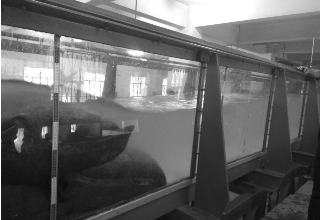
Figure 3(b): Data Collection in view (wave interaction with geotube)
