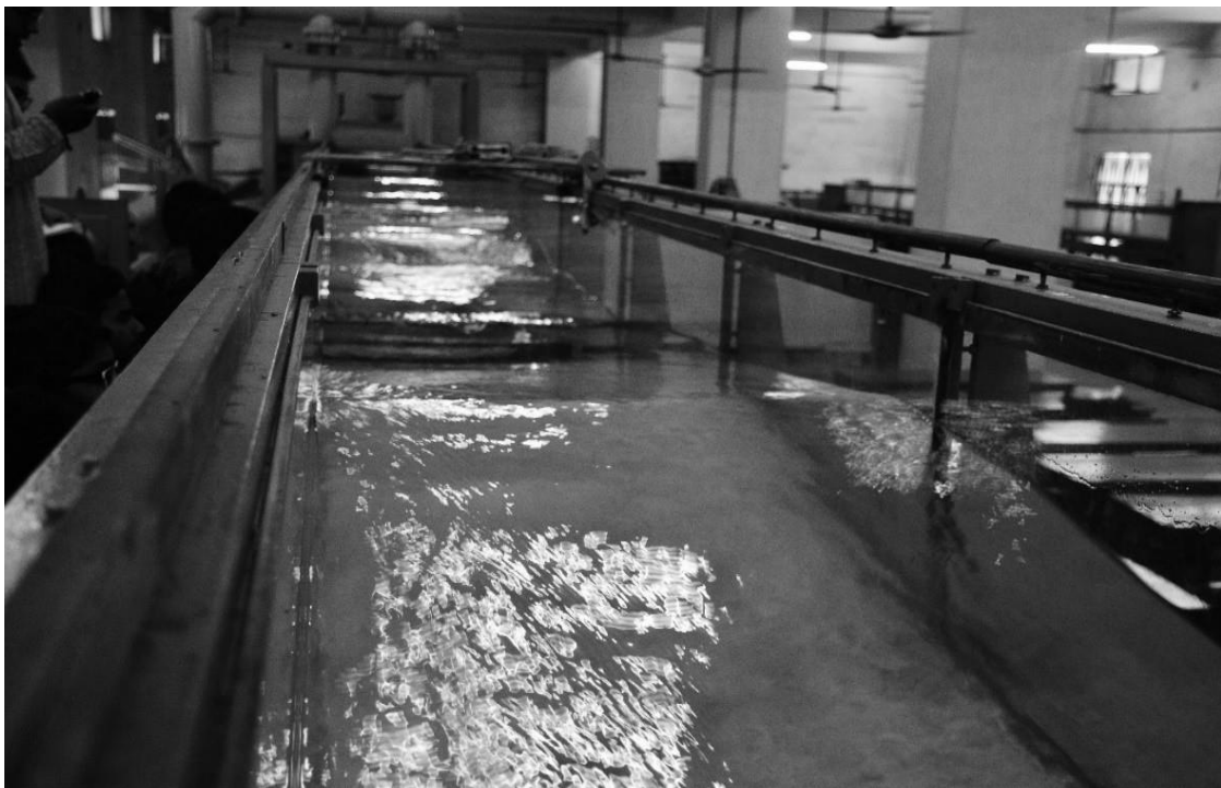
Figure 3(c): Data Collection in view (wave height reduction downstream)
