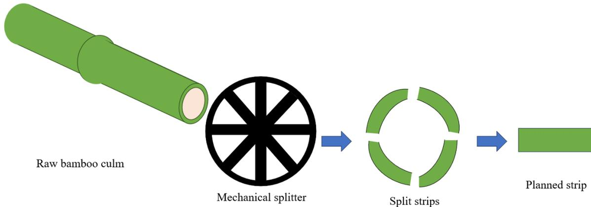
Figure 4: Steps to obtain planned strip for engineered bamboo production
