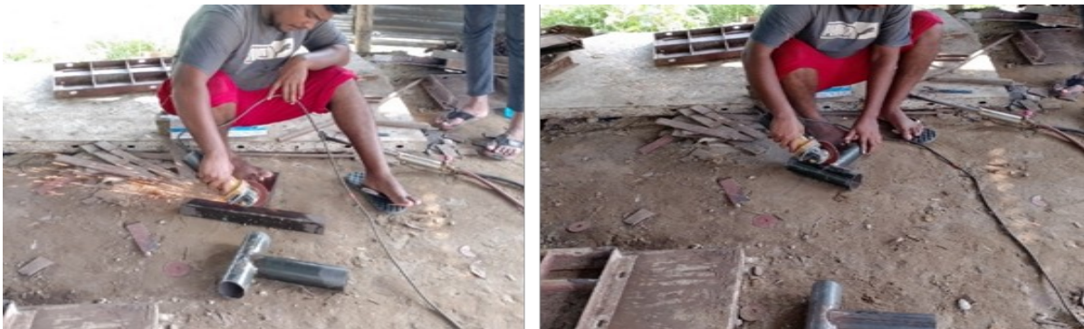
Figure 3: Cracking to make deficient T-joints by grinding machine
