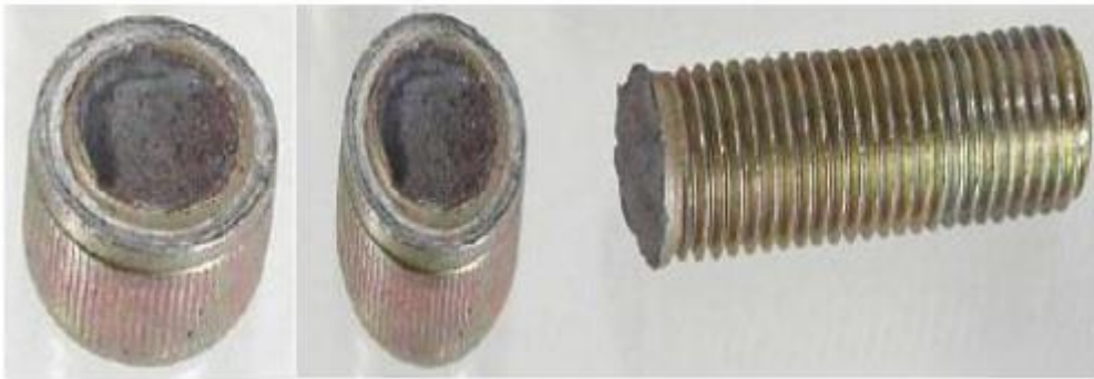
Figure 3: Typical Fastener Failure by Hydrogen Embrittlement (Ravinder & Deepak, 2014). The East Span of the Oakland Bay Bridge disastrous a test in 2013, six months before it opened. Shear bolts to the extent, experienced catastrophic disasters after just two weeks of use, which were attributed to embrittlement possibly caused by the environment (Khare et al., 2017).
