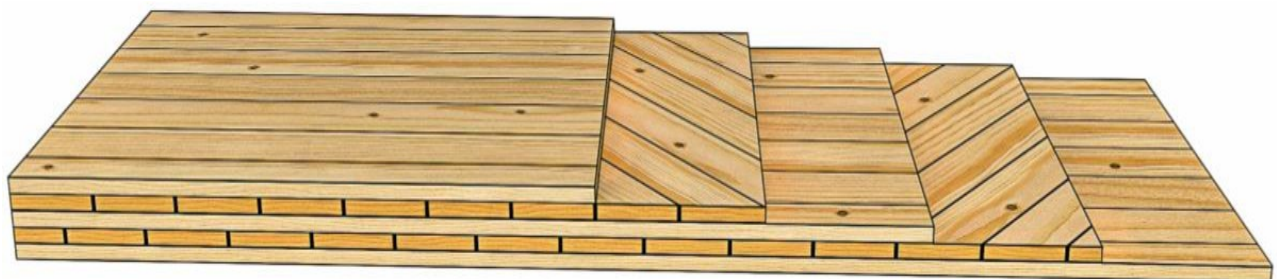
Figure 2: Angled ply CLT panel orientation detail
