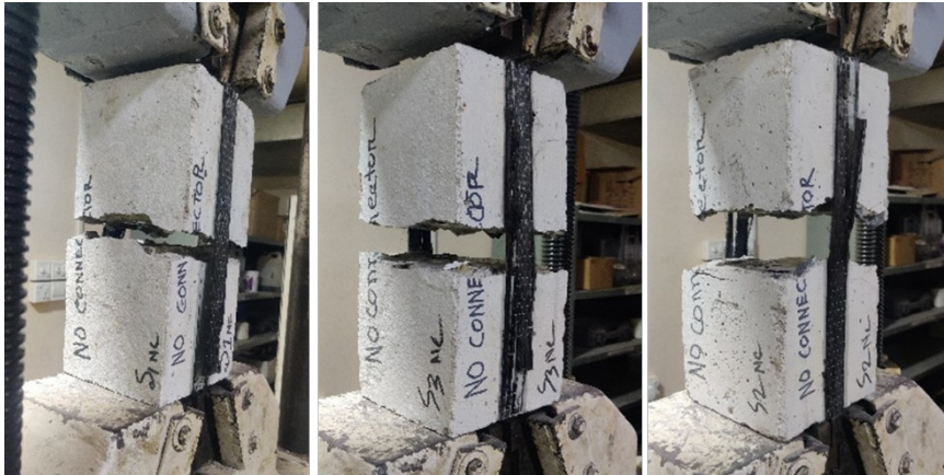
Figure 5: Failure modes of prism specimens without anchor.
