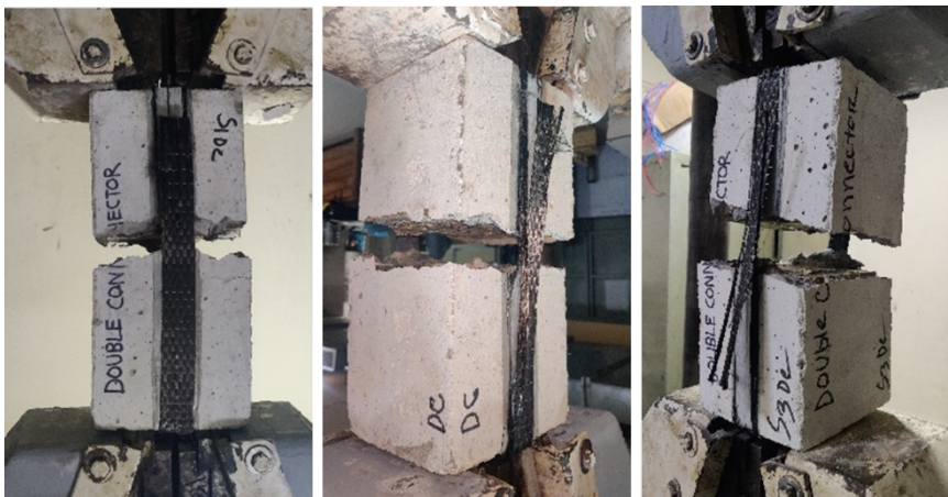
Figure 6: Failure modes of prism specimen with embedded double connector anchor.
