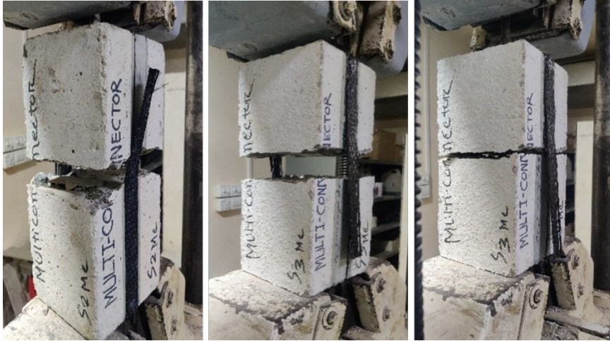
Figure 7: Failure modes of prism specimen with embedded multi connector anchor.
