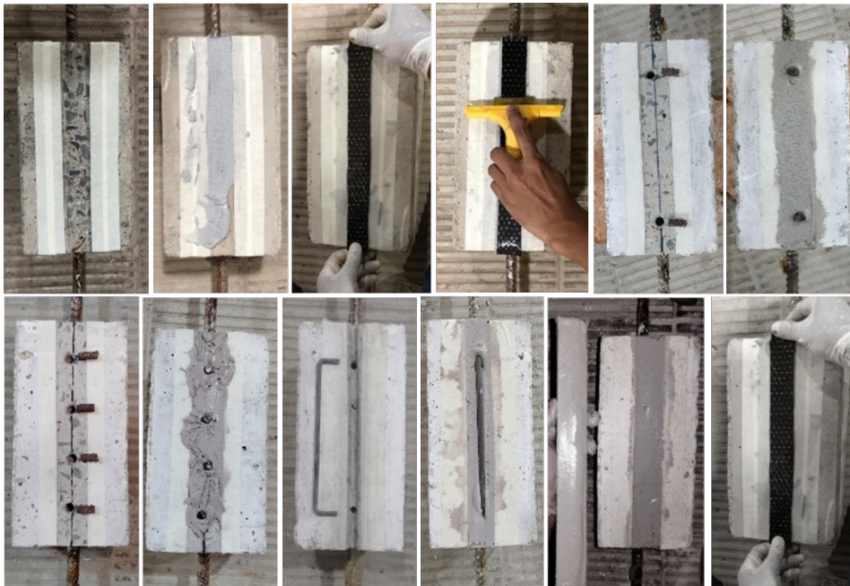
Figure 2: Strengthening process of RC prisms with CFRP wrap and anchors.
