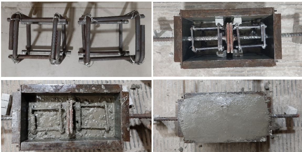
Figure 1: Reinforcement details and casting of prism specimens.
