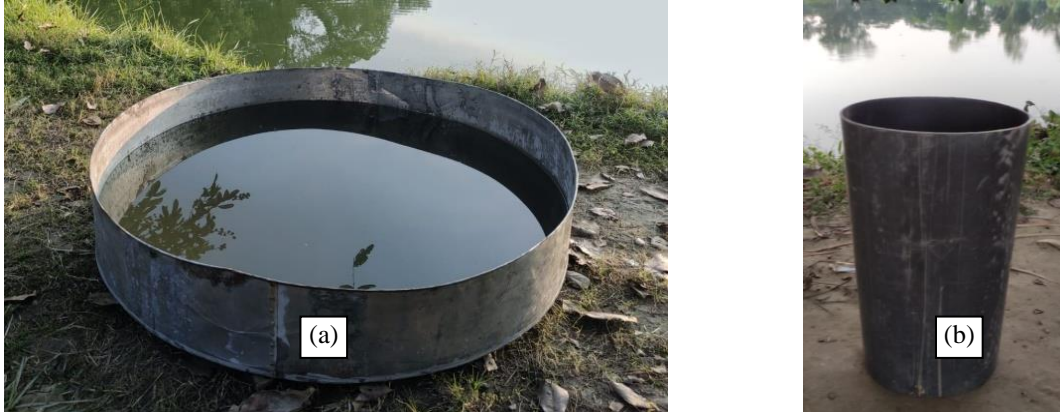
Figure 1: Water loss measurement instruments: (a) USWB class a evaporation pan, (b) Single ring infiltrometer
