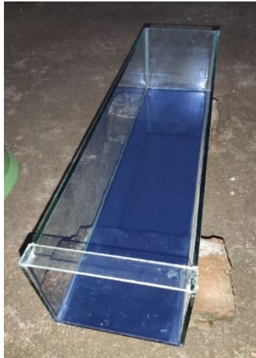
Figure 2: Glass made open channel drain
