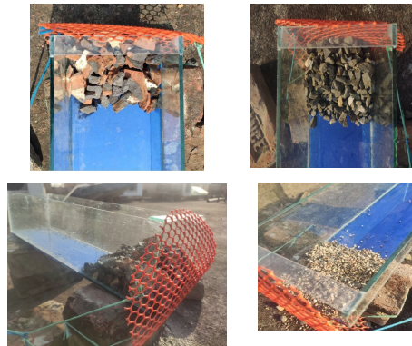
Figure 5: Various layers of a combination of materials to retain MP
