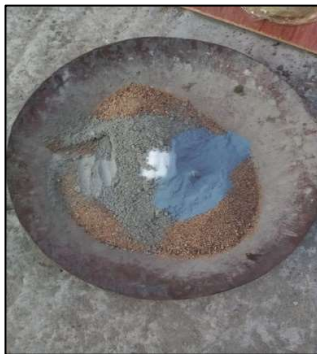
Figure 5: Addition of All Materials Except Water for Single Cylindrical Specimens
