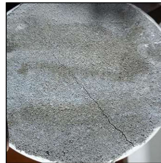
Figure 12: Formation of Cracks in Cylindrical Specimens.
