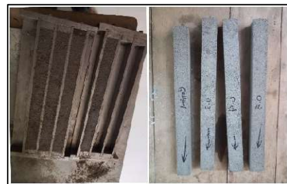
Figure 9: Casting and De-molding of Mortar Bars.
