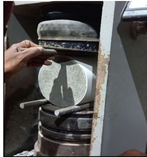
Figure 11: Inducing Lateral Load on Cylindrical Specimens.
