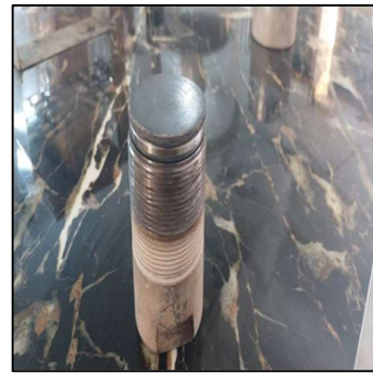
Figure 5: HTL Reactor with Copper Gasket and Steelhead
