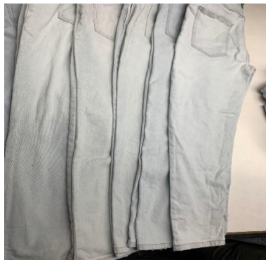
Figure 5: Denim jeans manufactured and washed using virgin caustic soda and treated groundwater
