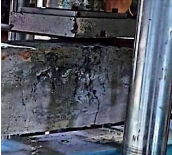
Figure 3.11: Failure pattern (for type 3 beam)
