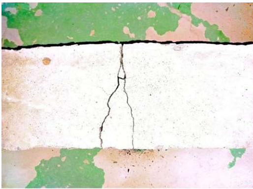
Figure 3.9: Failure pattern (for type 1 beam) Figure 3.10: Failure pattern (for type 2 beam)
