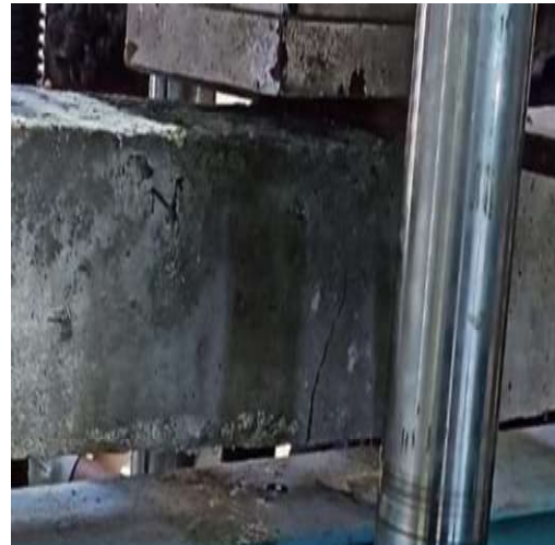
Figure 3.12: Failure pattern (for type 4 beam)
