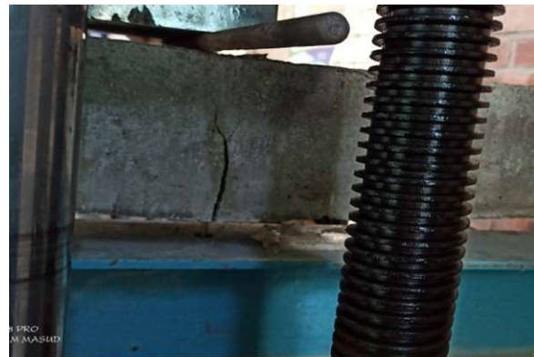
Figure 3.9: Failure pattern (for type 1 beam) Figure 3.10: Failure pattern (for type 2 beam)
