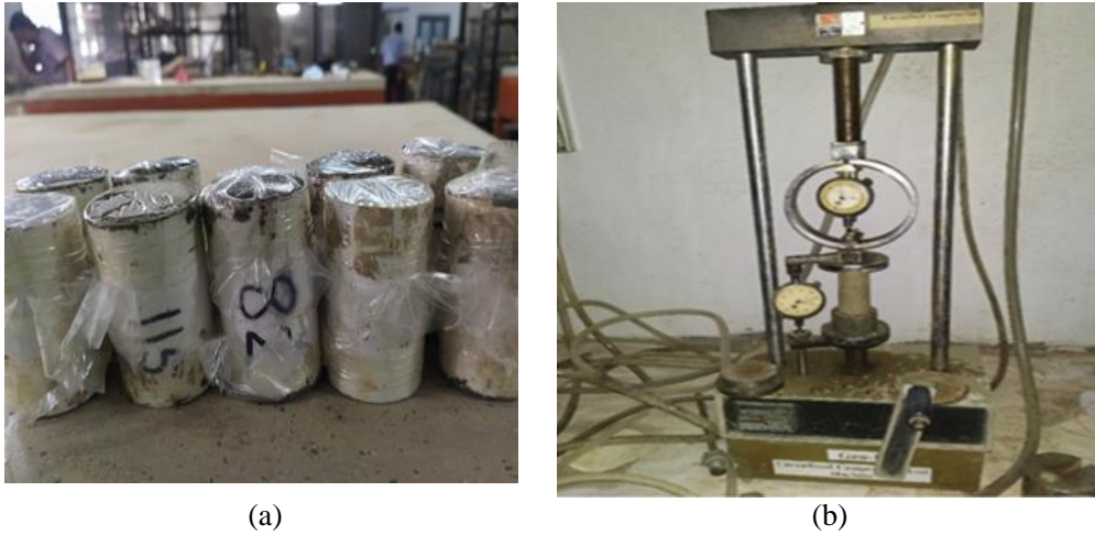
Figure 7: Cured sample before testing; (b) Sample is being tested on Unconfined Compressive Strength Testing machine
