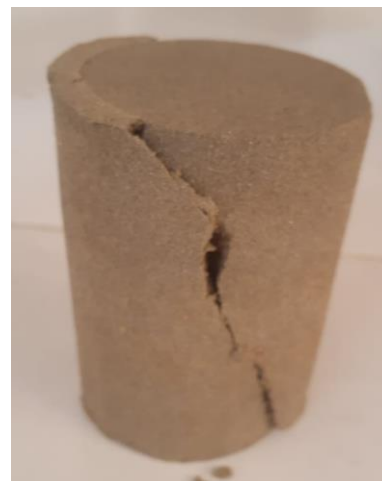
Figure 8: Testing the mould in UCS machine Figure 9: Failure pattern after testing the mould
