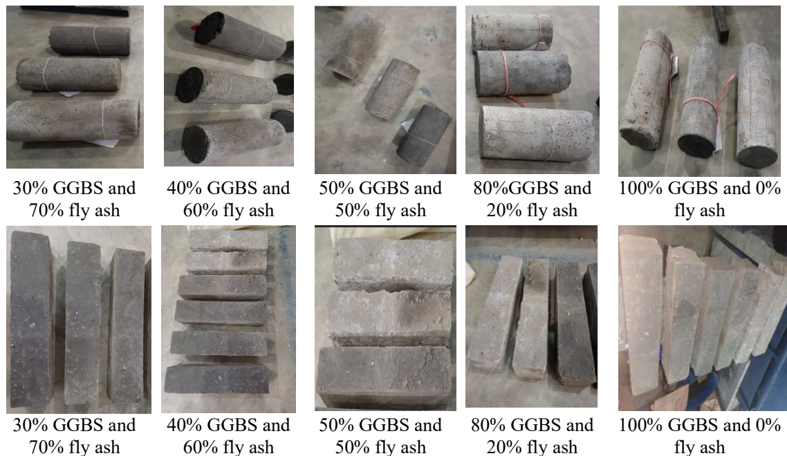
Figure 2: A visual representation of GPC and color in the curing process.
