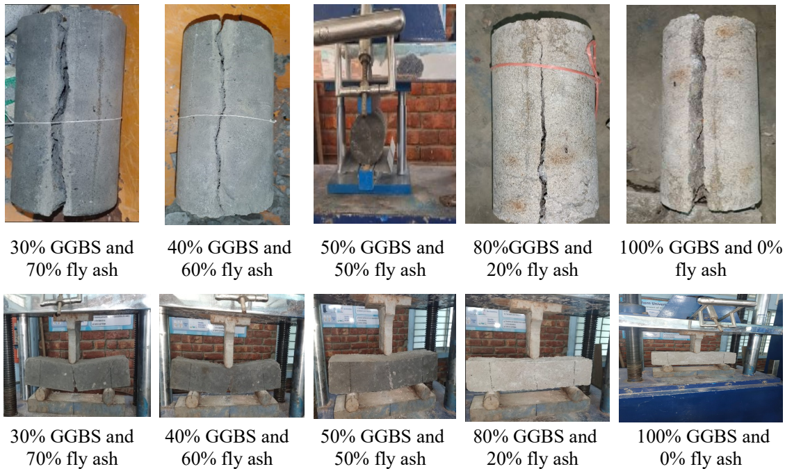
Figure 12: Failure modes of specimens.
