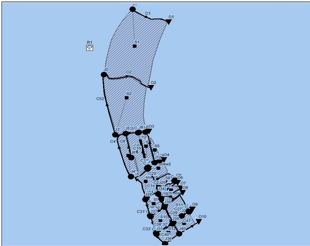
Figure 6: Model setup for water logging simulation in the study area in EPA SWMMv5.1 software
