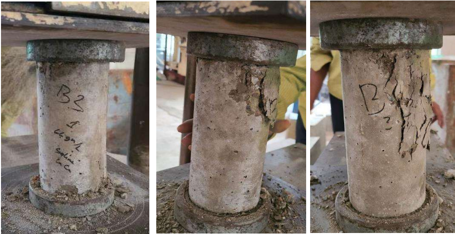
Figure 8 Compression Test of SS1 Batch for 7 days curing
