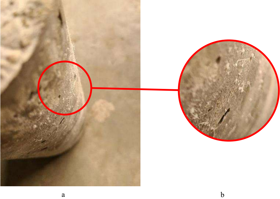
Figure 9 Salt deposit on SS1 Batch at 28 days curing
