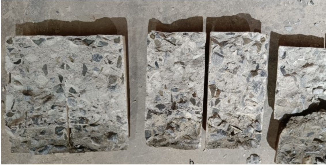
Figure 4: Water penetration in concrete specimens; (a)Ponding (b) Gunny Bag and (c) Air-cured
