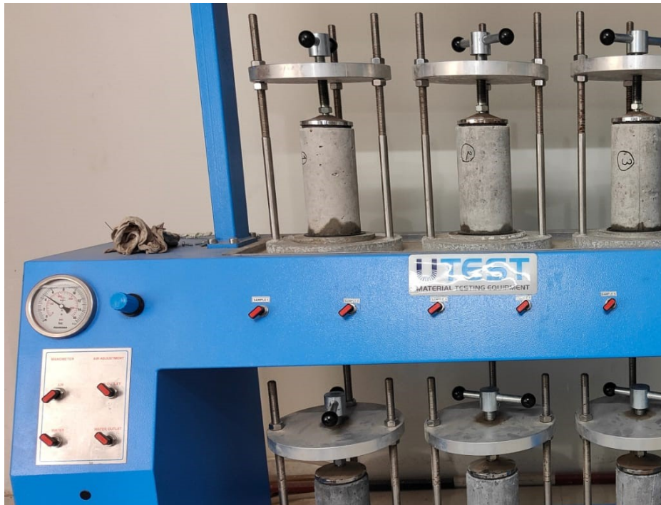
Figure 3: Water permeability test of concrete specimens
