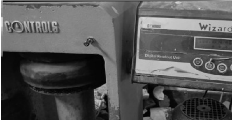
Figure 1: Compressive strength test of concrete specimen using CTM
