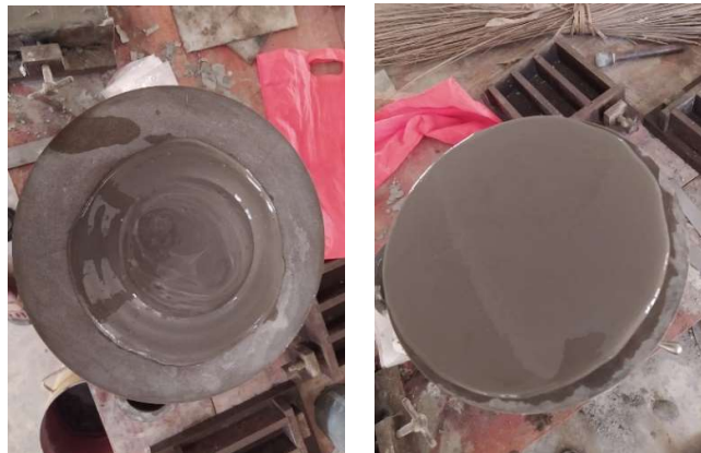
Figure 3: Flow Table Test
