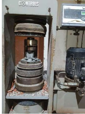
Figure 4: Compressive Strength Test
