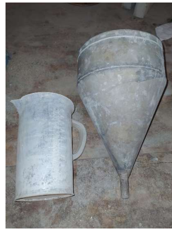
Figure 2: Flow Cone and Measuring Jar
