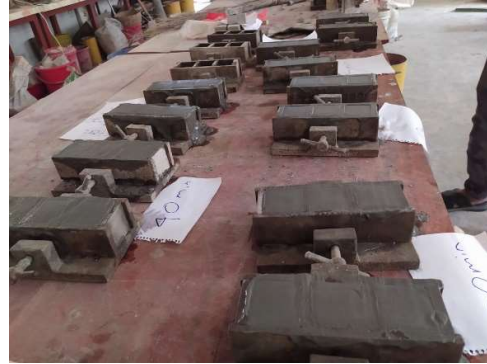
Figure 5: Preparation of Grout Sample
