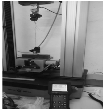
Figure 2: Tensile strength test using UTM
