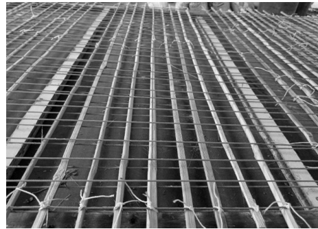
Figure 4: Preparation of Sample-2 & Sample-3 ( reinforced with bamboo and nylon)
