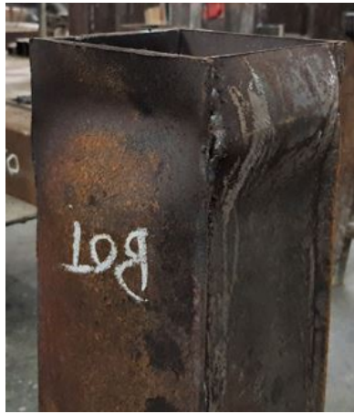
(a) Failure Pattern (Experiment)
